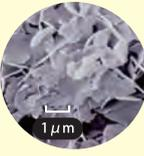
トバモライト<br>(11 Å Tobermorite)<br>$\text{Ca}_5(\text{Si}_6\text{O}_{18}\text{H}_2)(4\text{H}_2\text{O})$<br>結晶の形: 短冊状 |
